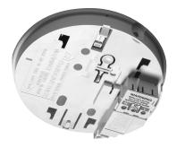
The primary function of the RadioLINK base is to interconnect all Alarms in the system, i.e. when one Alarm senses fire, the Ei168RC base attached to that Alarm will transmit an RF signal that will activate the sounders in all the other Alarms.
