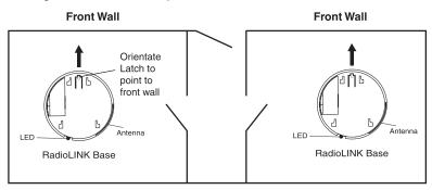
Orientate all RadioLINK bases in the same direction
