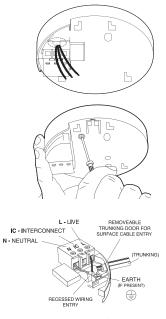
Slide the Alarm head onto the base. Connect the mains power to the alarm circuit.
