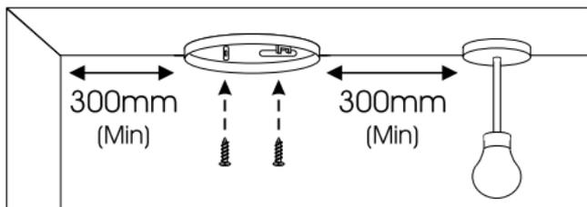
ALARM SHOULD BE CEILING MOUNTED AT LEAST 300MM FROM WALLS & OBSTRUCTIONS, IDEALLY CENTRALLY IN ROOM/AREA
