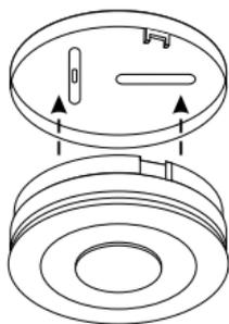
ON 10 YEAR LITHIUM BATTERY ALARM MODELS - TWISTING THE UNIT ON TO THE BASE AUTOMATICALLY CONNECTS THE BATTERY
