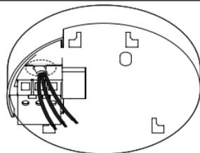
Screw the base to the ceiling using a single screw for now. The second screw should be inserted at the end of this procedure to secure the base permanently.
