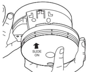
If the blue light flashes every 10 seconds, remove the alarm and manually depress the rechargeable cell "on" switch as shown and refit the alarm. If there is still a problem the cells may be depleted so leave the unit on mains power for 2 hours to charge and test again.
