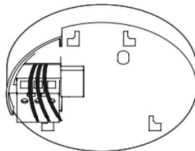
If the mains wires are being brought along the surface, break the knockout and trim to accommodate the conduit.
