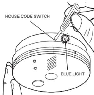
Check the communication by pressing the test/hush button for up to 20 seconds on each unit in turn. The red light will flash, the Alarm will sound and blue light on the RadioLINK Base sidewall will illuminate continuously for around 3.5 seconds. All other Alarms should sound (this may take up to 20 seconds).
