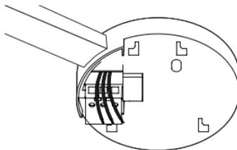
To prevent air draughts affecting smoke or heat entering the alarm it is important to seal the area around the hole in the ceiling with foam or silicon rubber.
