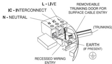
Slide the Alarm head onto the base. Connect the mains power to the alarm circuit.
