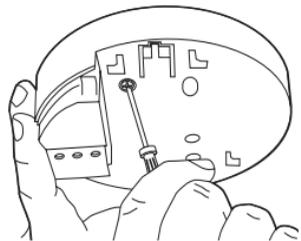
Slide Alarm on to the Ei168RC RadioLINK Base. This will automatically activate the rechargeable back-up cells in the base.
