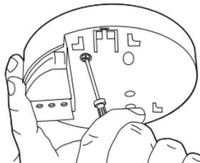
Connect the wiring to the terminal block as shown here.
