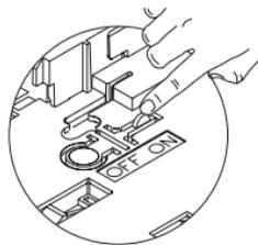
Press and hold the test button. The red led will flash and the horn will sound.
