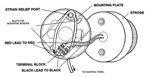
MOUNTING PLATE TO BE FIXED TO WALL AS SHOWN FOR ROUTING THE CONTROL PANEL CABLE DOWNWARDS
